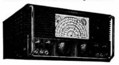
Fifteen valves; 5 bands, 480 kc/s,-30 Mc/s.; precision tuning free of backlash; fine logging scale; accurate calibration; 2 R.F. stages; crystal filter; stabilised oscillator; true variable selectivity; effective noise limiter; "S" meter; push-pull quality output.
